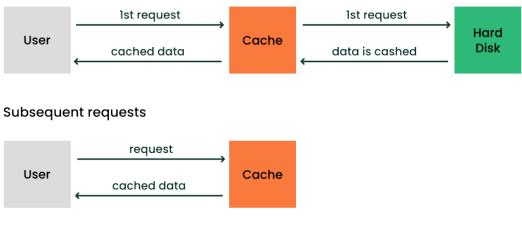
FIGURE 16.1: CACHING MECHANISM
